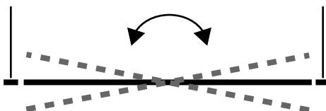
**15** To adjust the position of the diffuser, rotate it by holding the heads /
