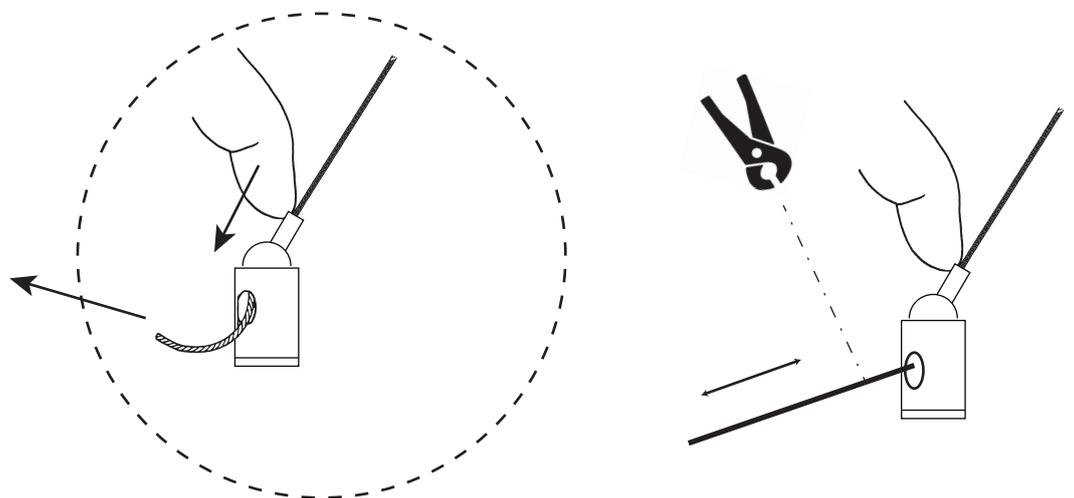
5 Place the pole into the holder. Start with the cable. **5A** Fix the pole by tighten the two screws
