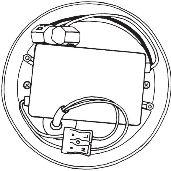
10 Connect the wires to the two terminal clamps and pay attention that the polarity is correct.
