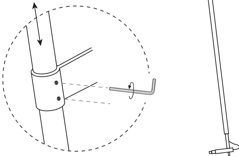
**6** Assemble the tapered rod / Screw the tapered rod into the lamp pole.
