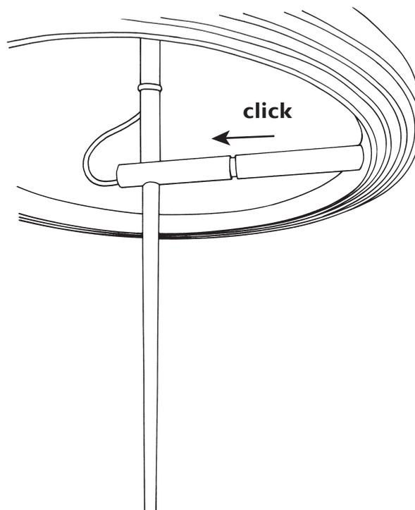
8 The telescopic fitting is adjustable by up to 60 cm
