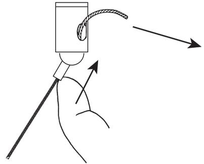
lift the disc by using white handcloves and insert the cable into the cable holder.
