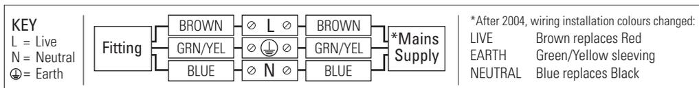
9. Double check all the connections are secure and that no loose strands of wire are left out of the connector. Ensure the lid of the terminal block is closed securely after making the connections.
