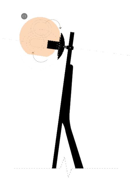
/ C1 is fixed on C5 by twisting the globe through the cut out on C5 / C1 needs to sit neatly on C5  $\,$
